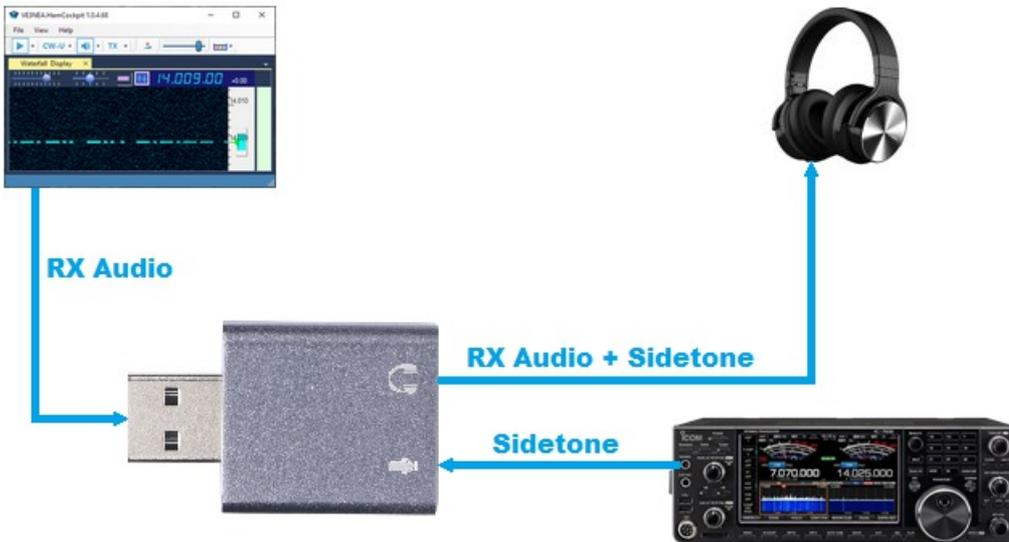
The sidetone may come from the Morse keyer or, if the keyer is built into the radio, from the Phones connector of the radio (but not from the ACC connector). Make sure that only the sidetone is present and receiver audio is muted. How to achieve this is radio-dependent: for example, in TS-570 you can set the IF gain to the minimum, and in IC-7610 you just press the Main AF knob.
